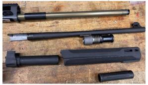
3: Install the supplied Briley piston stop sleeve over the magazine tube with the "winged" end towards the receiver. It is easiest to put the piston stop against the gas piston and install both the barrel and piston stop together.
