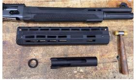
2: Start by locking the bolt to the rear and removing the factory barrel, magazine clamp, magazine cover, and forend per the owner's manual. Do not close the bolt during installation
