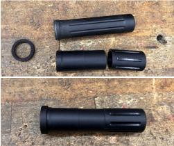
5: Once the ring and piston stop are installed, the gun can be assembled as normal, replacing the factory forend with the Briley M-Lok Handguard. First slide the handguard over the barrel and magazine tube until it seats against the receiver. The handguard will be stiff to seat completely over the piston stop at first. This is due to a detent that keeps the piston stop from riding forward, and is normal. Please note it will also be tight when removing the handguard from the barrel.
